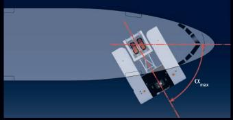
Models with an oversteering protection system measure the forces and avoid damage to the nose gear.
