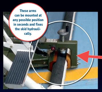
The HELIMO moves every type of helicopter with skids regardless of obstacles such as cameras, radar, floats, winds and weapons mounted on the belly or skids of the helicopter. The HELIMO is universal and easily adjustable to meet the specifications of the helicopter.
