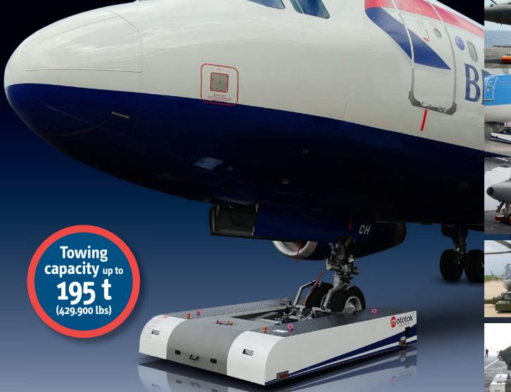
• Easy hydraulic wheel adjustments for different wheel sizes.
